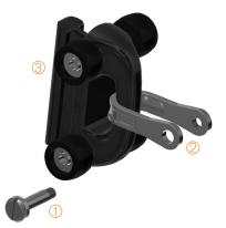
1. Detach the pin ① from the shackle and insert the shackle bow ② into an applicable Rutgerson Pressure Absorbing Slide ③ (not included in the 1529 kit).
