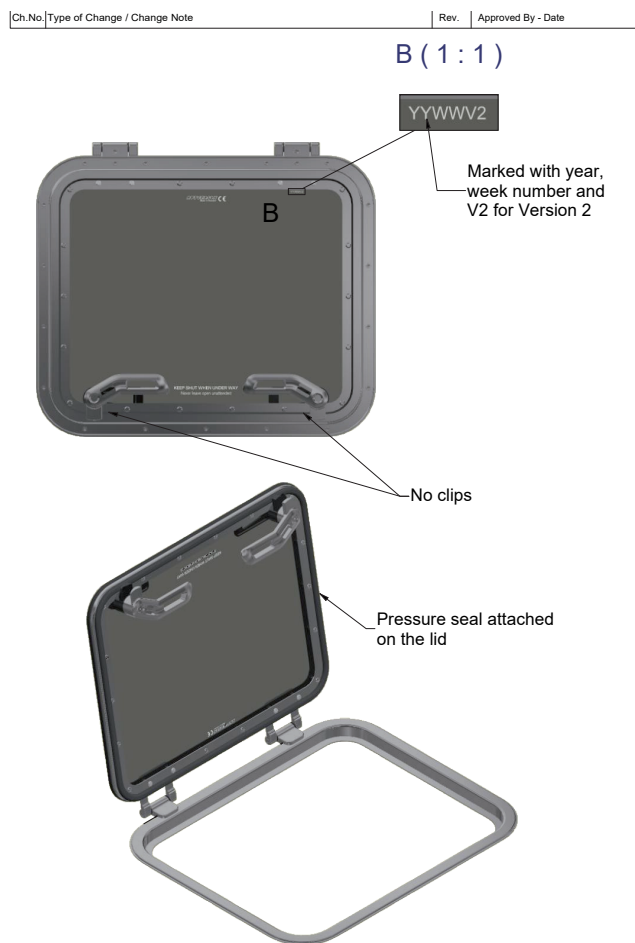
Multihull Escape Hatch H2255-5400 Version 2, from April 2021
