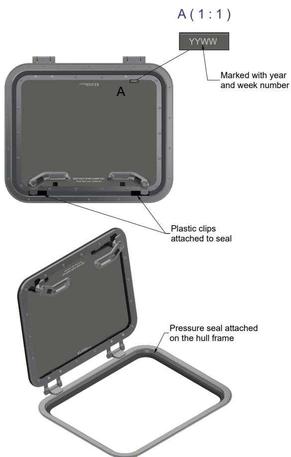
Multihull Escape Hatch H2255-5400 Version 1, until March 2021
