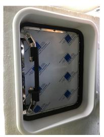
3. Attach the end piece to the bar. Place the locking bar in the spaces of the two handles and slide the spare part onto the stainless steel handle.
