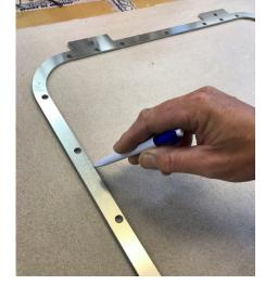
2. Cut the hole for the hatch in the hull and then drill all 22 holes with a 9 mm drill through the hull from outside
