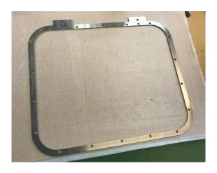
1. Place the cutout template on the hull exactly where the Escape Hatch should be located. Mark with a pen on the inside of the template where the cutout hole will be as well as the 22 screwholes.
