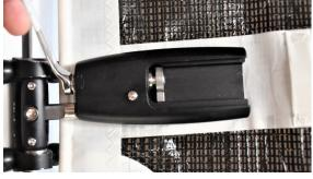
Turn the tensioning bolt clockwise to release the tensioning plate. Don't stop until the plate reaches its most opened position.
