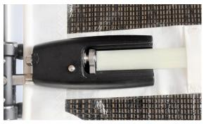
4. Make a straight cut at the mark and reinsert the batten. It should fit snugly between the batten pocket and the released tensioning plate.
