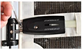
6. Adjust the tension as needed by turning the tensio ning bolt anti-clockwise. The window in the lid will help you to keep track of your trimming.
