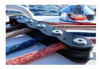
Like all our other products these organisers are designed and manufactured in our factory in Marstrand, Sweden. Both sides and sheaves are made of black hardcoat-anodized aluminum and shall be fitted with M12 countersunk head screws (ISO 10642 or DIN 7991) with a maximum head diameter of 24mm. Screws are not included, and shall be chosen depending on deck thickness. Optional mounting plate is available as spare part.
